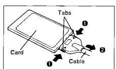
Pull the cable while pressing the side tabs of the cable
